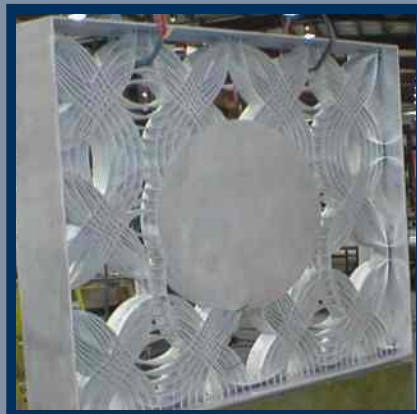
An example of a water jet piece cut from a solid 4" thick chunk of aluminum for use as a decorative structure. Designed by Sussman/Prejza & Company Inc.
