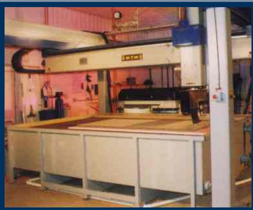
5-Axis Single Head Water Jet Cutter
