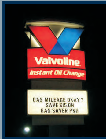
Valvoline ~ Woodbury, MN The V is thermal formed and backed with translucent vinyl and back-sprayed white. The Valvoline letters are embossed and backed with translucent red vinyl and back-sprayed white.
