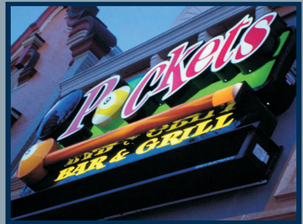
Pockets Bar & Grill ~ Fond Du Lac, WI Billiard ball faces and pool cue are thermal formed polycarbonate with digital prints applied 2nd surface.
