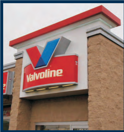
Valvoline ~ Woodbury, MN The V is thermal formed and backed with translucent vinyl and back-sprayed white. The Valvoline letters are embossed and backed with translucent red vinyl and back-sprayed white.
